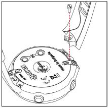
b) Remove the two screws near the padlock symbols. These hold the battery cover in place.
