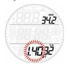
This leads you to the **G2 OFF** screen. Press and hold the lower button to exit the menu or go to section 3.5 for information about diving with more than one gas.
