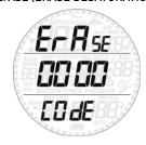
Smart allows you to reset the desaturation in the computer. Any tissue saturation information from a recent dive will be reset to zero and the computer treats the next dive as a non-repetitive dive. This is useful when the computer is loaned to another diver who has not dived in the last 24 hours.
