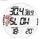
In this case, if the diver attempts a repetitive dive after surfacing, Smart will only function as a depth gauge and timer (bottom timer mode), and will display **DOWN!** on the screen throughout the dive.
