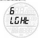
Smart has a backlight which can be activated in case of low ambient light. The backlight is activated by pressing and holding the lower button. During a dive, the backlight will stay on for the duration defined in this menu. You can choose between 1 and 10 seconds.
