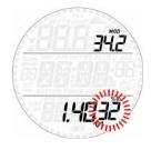
Once inside this menu, press either button to change the  $0_2^{\, \%}$  and observe how this affects the maximum operating depth (MOD). Then press and hold the upper button to move on to the pp $0_2$ max and use either button to change the value, again noticing how this affects the MOD. Press and hold the upper button again to save the setting.
