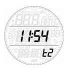
Smart features a "sleep" mode: in case you don't wear it other than on a dive trip, you can put Smart in sleep mode to reduce battery consumption. To wake up from sleep mode, press either button.
