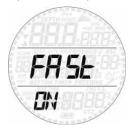
A fast (uncontrolled) ascent is defined as one in which a speed of 12 m/min / 40ft/min or higher was maintained over more than two thirds of the way up. This applies to dives deeper than 12m/40ft only. In such an event, due to the potential of harmful bubble formation, Smart locks the computer for 24 hours in order to discourage you from diving again. In this menu,
