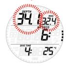
The alarm persists until the diver has ascended enough for the  ${\rm ppO}_2$  to return within the set limit.
