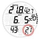
Press the upper button while this indication is blinking to initiate the gas switch: the oxygen percentage of G2 starts to blink in lieu of that of G1, and in the top right corner the letters MOD and the value of the MOD for G2 appear, blinking.
