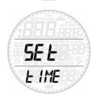
Press and hold the upper button to enter a menu, then press either button to scroll up and down between available options or to increase or decrease the value of a setting. Then press and hold the upper button to confirm the change in setting. Press and hold the lower button to go up one level in the menu tree.
