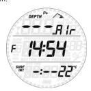
The pre-dive display shows p factor and altitude settings, time of day, surface interval since the last dive and temperature. If Nitrox is set, it will show the  $\rm O_2$  percentage and the corresponding MOD. A small S or F to the left of the middle row indicates the water type.
