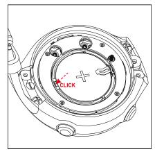
g) Position the new o-ring from the kit in the groove around the battery, ensuring that it sits towards the outer edge of the groove.
