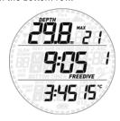
Press and hold the upper button to enter the session and see max depth and sequential counter of the immersion at the top, dive time in the middle, surface interval prior to immersion and minimum temperature of the immersion at the bottom.
