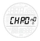
Press and hold the upper button to enter this menu. The middle row now features a stopwatch while the time of day has moved to the bottom row. Press the upper button to start and stop the time, then press the lower button to reset the time to zero. Press and hold the lower button to exit from the stopwatch function (this stops and resets the stopwatch if it was running or stopped at a non-zero value upon exiting).
