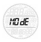
Here you can define the type of gas you will be breathing during the dive (air or enriched air nitrox, including multigas). You can also set Smart to bottom timer, in which case Smart will show only time, depth and temperature: it will not carry out any decompression calculation and it will not show any warnings and alarms. You can set Smart also to freediving mode, which in essence is a bottom timer with special features dedicated to free divers
