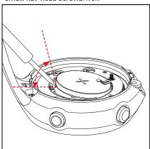
f) Replace the battery with the new one from the kit. The battery should click in place. Make sure to respect the correct polarity of the battery: the "+" has to be facing outwards.
