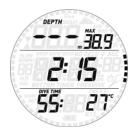
Upon returning to the surface, Smart first goes into the so-called surfacing mode. This mode allows you to resume your dive after a brief period of orientation. The screen shows a 3-minute countdown.
