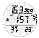
For **DECO** stops, since the duration is a function of the exact depth, only the minutes are shown.
