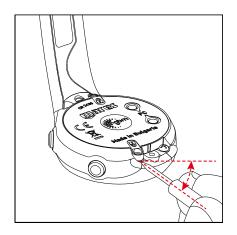
d) Remove the cover then remove the o-ring.
