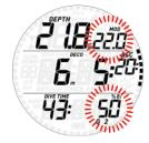
Press and hold the upper button to confirm the switch to G2, or press the lower button to cancel the gas switch and stay with G1. In both cases the set oxygen concentration will be displayed steadily in the lower right corner of the screen, and within 20 seconds the ascent time is updated to reflect the higher oxygen concentration in the breathing gas.
